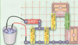
If the loose ends of the jumper wires are placed into a cup of water, the LED will be dimly lit. The circuit was designed so that the LED acts as a water detector. The brightness depends on your local water supply. If more water were added to the cup, the LED brightness would increase slightly. Adding more water is like placing more "water resistors" in parallel; and so decreases the total
