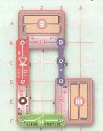
The brightness of the LED depends on how much light shines directly on the photoresistor. If the photoresistor were held next to a flashlight or other bright light, then the LED would be very bright.
