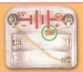
This thermistor will activate to limit current if a short circuit occurs for more than a few seconds. Running the motor for long periods will sometimes activate it, since the motor draws a high current.
