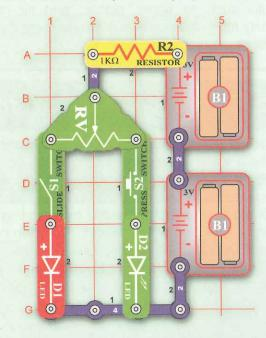
If the slide switch and the press switch are both on, moving the adjustable resistor's control lever around will adjust the brightness of the LEDs. When the adjustable resistor is set to one side, that side will have low resistance and its LED will be
