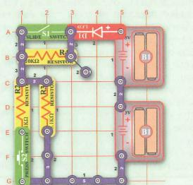
If the slide switch (S1) is on, then the LED will be on but not very bright as the 5.1K resistor limits the current. Turning off the slide switch places the 10K resistor in series and the LED becomes very dim. If both switches are on, the 1K resistor is in parallel with the 5.1K and so the LED becomes very bright.
