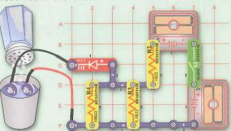
Dissolving salt in water decreases the resistance of the water, so the LED would get brighter. It could be used as a salt-water detector. Adding more water to dilute the salt could reduce the brightness.
