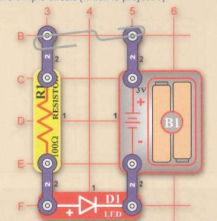
Place any material across the 2-snap wires (the circuit shows a paperclip). If the LED is bright then it is a conductor, if the LED is off then it is an insulator.
